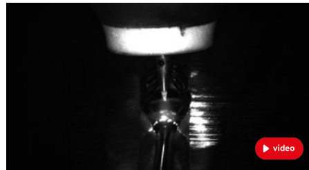
NARROW GROOVE WELDING (SAKKY FINLAND)
