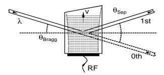
An AO device works through the interaction of sound (RF) and light. This is achieved via a piezo-electric transducer bonded to one face of a suitable crystalline material. When an RF drive signal is applied to the transducer, a <u>travelling</u> acoustic wave is produced in the crystal. This creates areas of compression and rarefraction, similar to the slits in a diffraction grating.
