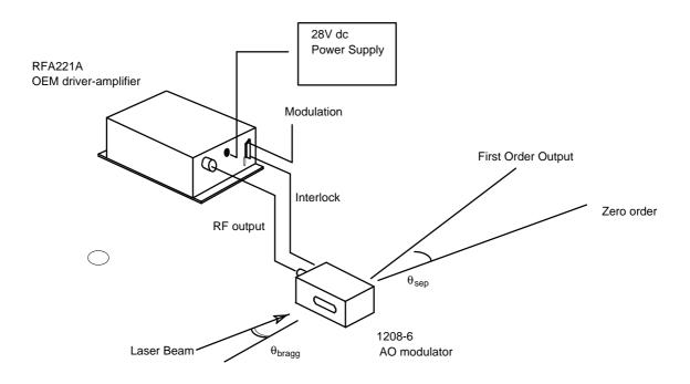
The input Bragg angle, relative to a normal to the optical surface and in the plane of deflection is:
