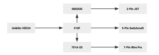
This graphic (left) shows how the VED24 should be interfaced with various shutters devices/shutter connectors using the included adapters and interconnect cable.
