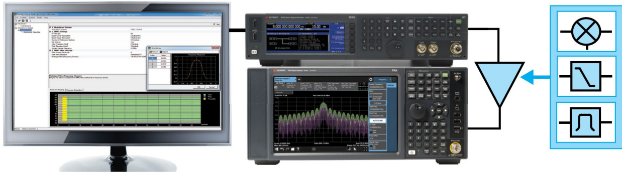
Figure 8.2: Typical component test configuration using Signal Studio with an X-Series signal generator and analyzer
