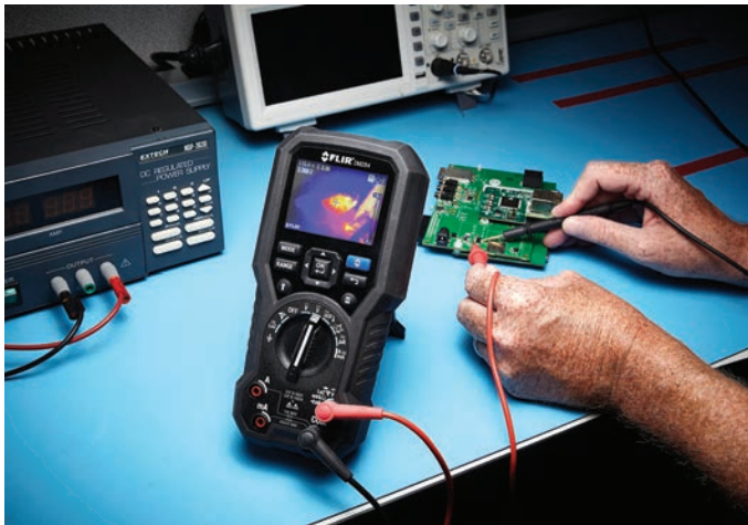
All-in-one meters with integrated thermal imaging allow for fast inspections of electronics systems
