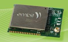
**EMB-LR1272E** is a powerful OEM sub-1GHz wireless module featuring the Semtech LoRa long range modem providing ultra-long range spread spectrum communication and high interference immunity on the 868/915 MHz radio band. It embeds a full LoRaWAN Class A and Class C protocols enabling connection to any LoraWAN compliant network infrastructure.
