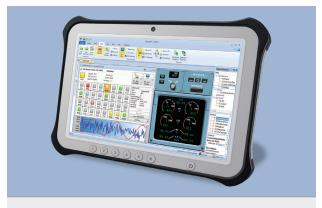
CoPilot is an intuitive, graphical software program that allows you to easily monitor, record, replay, analyze, and simulate avionics bus data, and interact with data directly on multiple buses using interface hardware.
