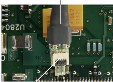
ZIF tip soldered to target
