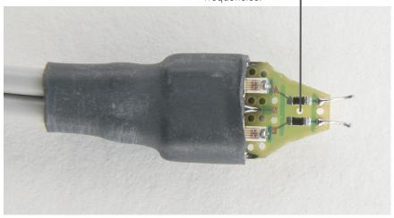
Figure 2. InfiniiMax solder-in probe head detail
