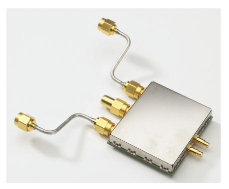
Figure 8. N5380A dual-SMA differential probe head
