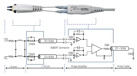
Figure 1. InfiniiMax architecture
