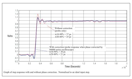
Figure 3. Time domain response of N5381A solder-in probe head and 1169A probe amplifier  $\,$
