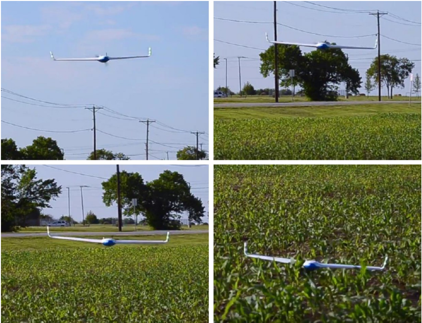
Figure 4 – Various altitude-dependent steps are performed during the Eclipse's approach and landing phases to ensure a smooth glide to the ground
