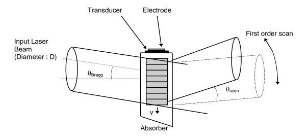
The diagram depicts an acousto-optic deflector showing the sound column, of frequency f , travelling at velocity V through the AO crystal. The straight through zero order beam is not shown for clarity.
