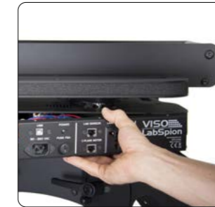
The main board easily slides into allowing a quick update
