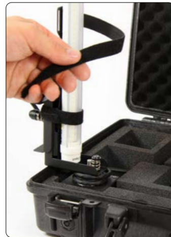
A linear lamp bracket is included to measure long light sources, get lumen per meter or per foot.
