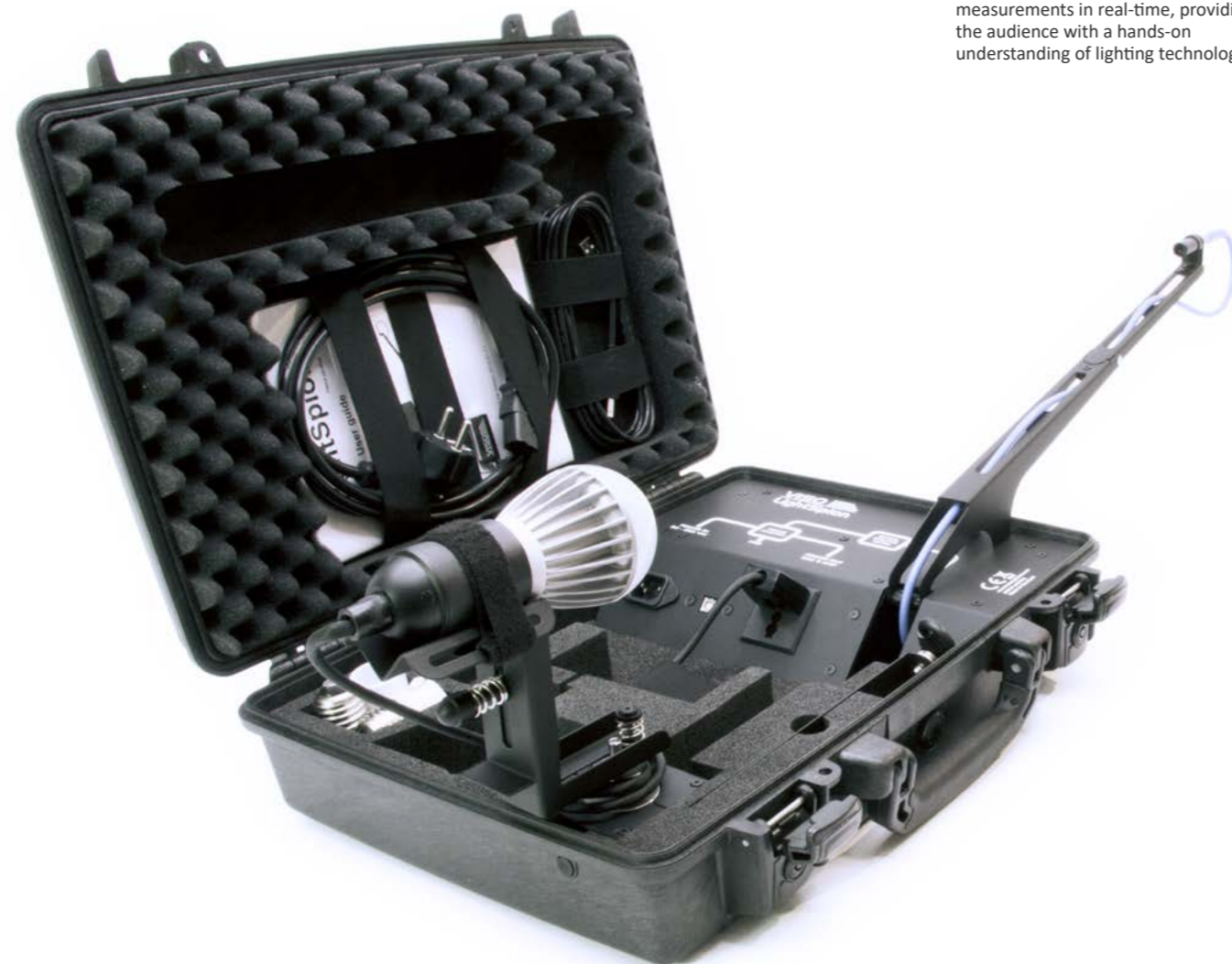
A linear lamp bracket is included to measure long light sources, get lumen per meter or per foot.
